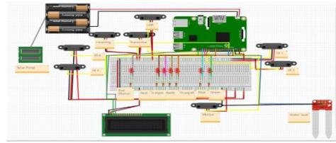
the drivers about it, LEDs also will serve the same purpose, Red is when all sensor is detecting, yellow if one, Blue is when the water level is high, and green is when the light is detected. SBC is connected to the power supply and also to WiFi. The SBC connects to the monitor using an HDMI cable and also to the USB keyboard and mouse. To the different GPIO pins, we connect different sensors and actuators.
