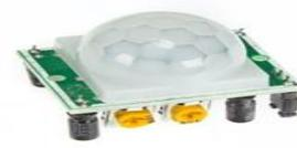
Figure 6: Motion sensor
