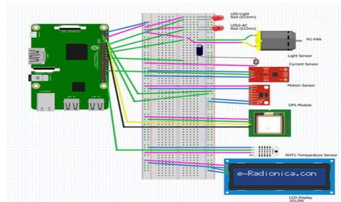
Figure 11: Proposed System Circuit Diagram
